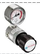
Line regulator - Single stage Mounting on pipe network, gas panel or point of use Suitable for pure gases and mixtures, non corrosive Made of stainless steel Working pressure from 0,05 to 10 bar. Flow rate up to 3, 5Nm<sup>3</sup>/h
